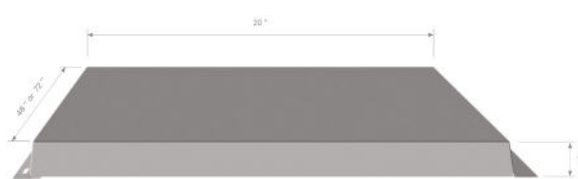
Panel 20 x 48 x 1 in Panel 20 x 72 x 1 in Panel 20 x variable length x 1 in
